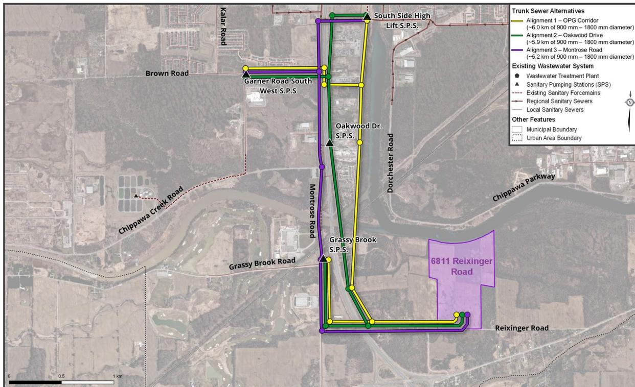
Figure 5-6. New SNF Trunk Sewer Alternatives
