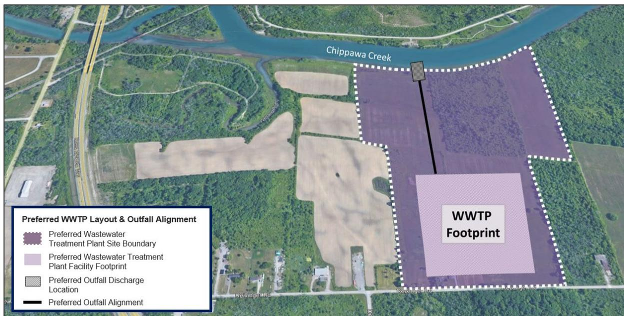
Figure 6-1. Preferred South Niagara Falls Wastewater Treatment Plant Site
