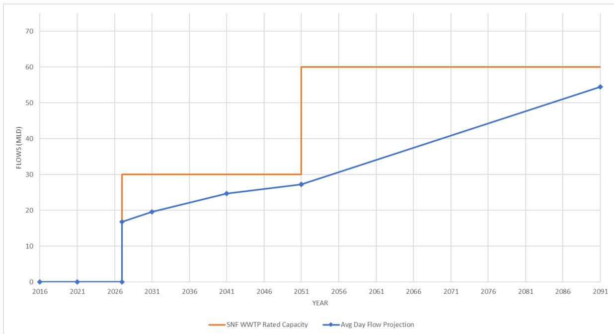
**Figure 5-2. New South Niagara Falls Wastewater Treatment Plant Flow Projections**
