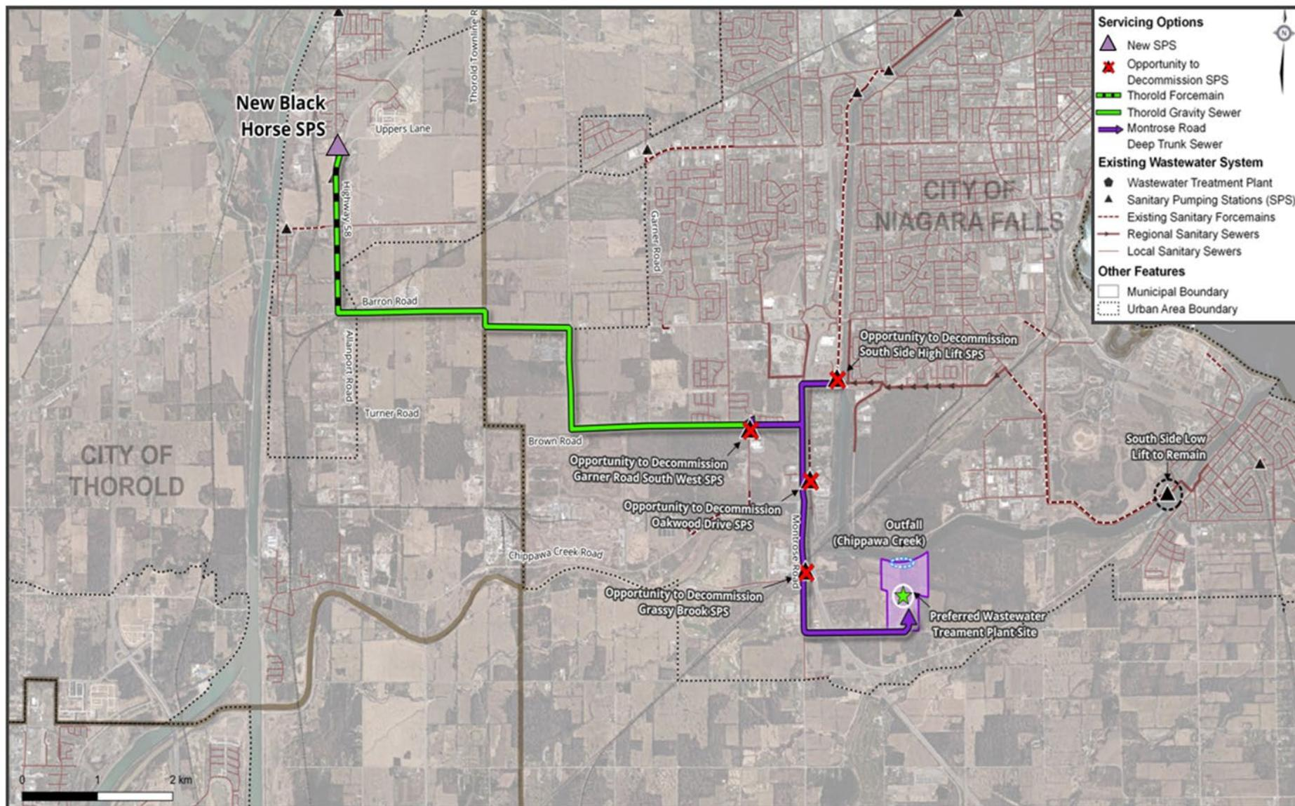
Figure 6-6. Preferred SNFWWS Integrated Solution and Design Concept
