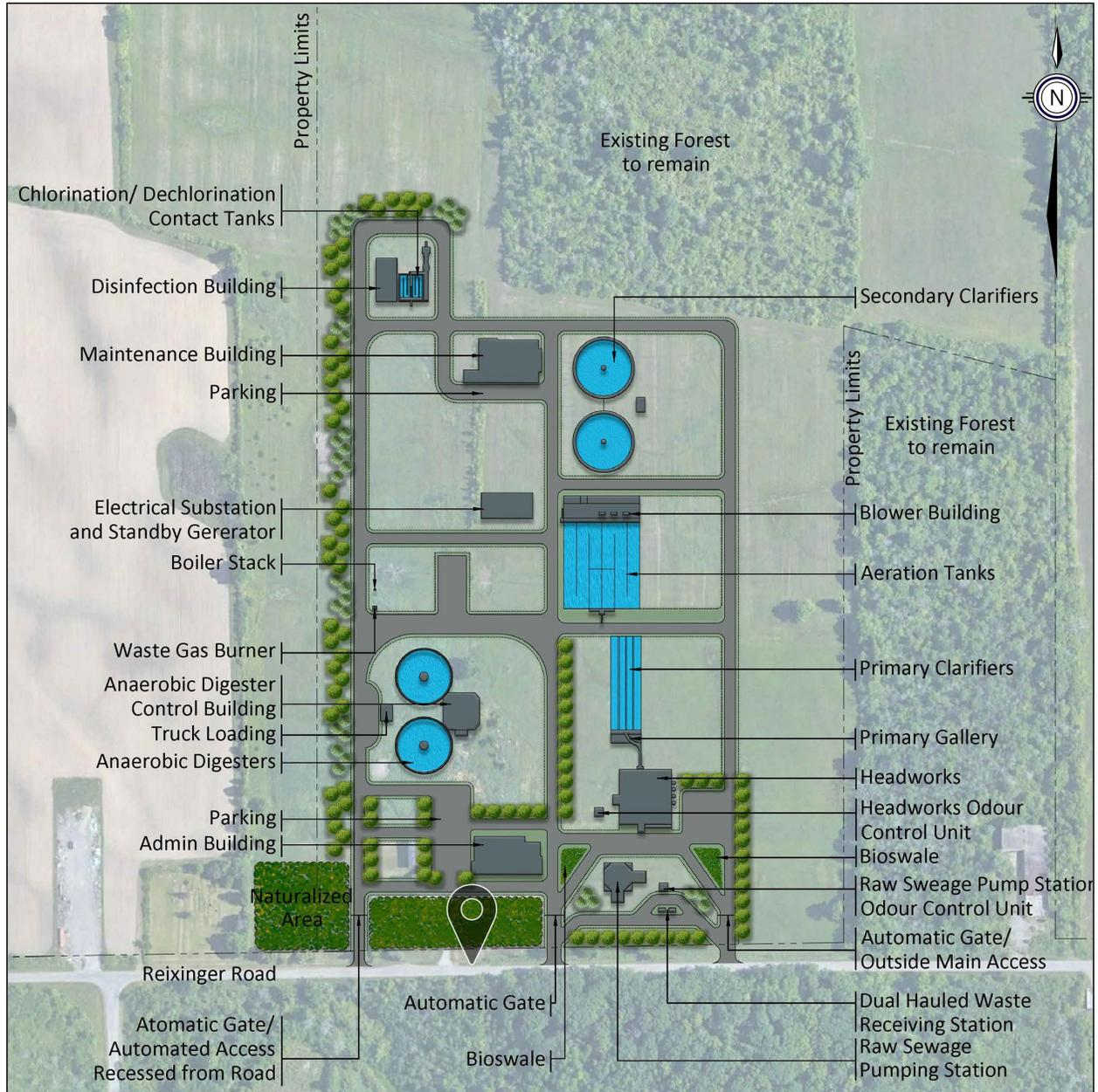
**Figure 6-2. Preferred South Niagara Falls Wastewater Treatment Plant Site Layout and Facility Locations**
