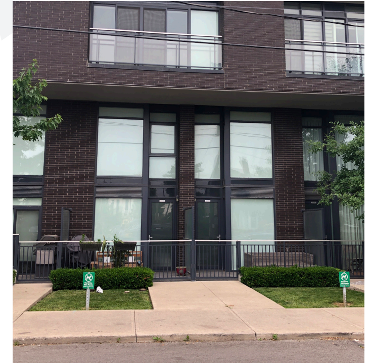
Figure 182: Two-storey townhouse units incorporated into a mid-rise form allow for privacy of bedrooms located at the second storey.
