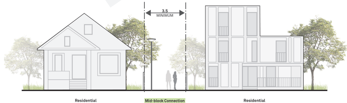
Figure 77: Residential mid-block connections should be at least 3.5 metres wide and include pedestrian-scaled lighting.
