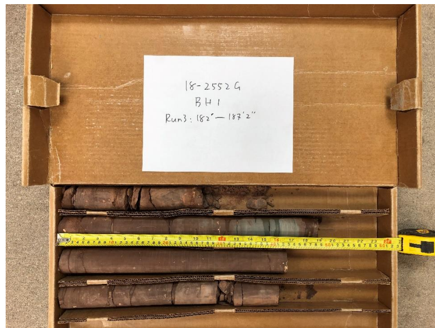
Photo 2: Borehole BH1 Rock Core Run 3: 182'0" – 187'2" (55.47 m – 57.05 m)
