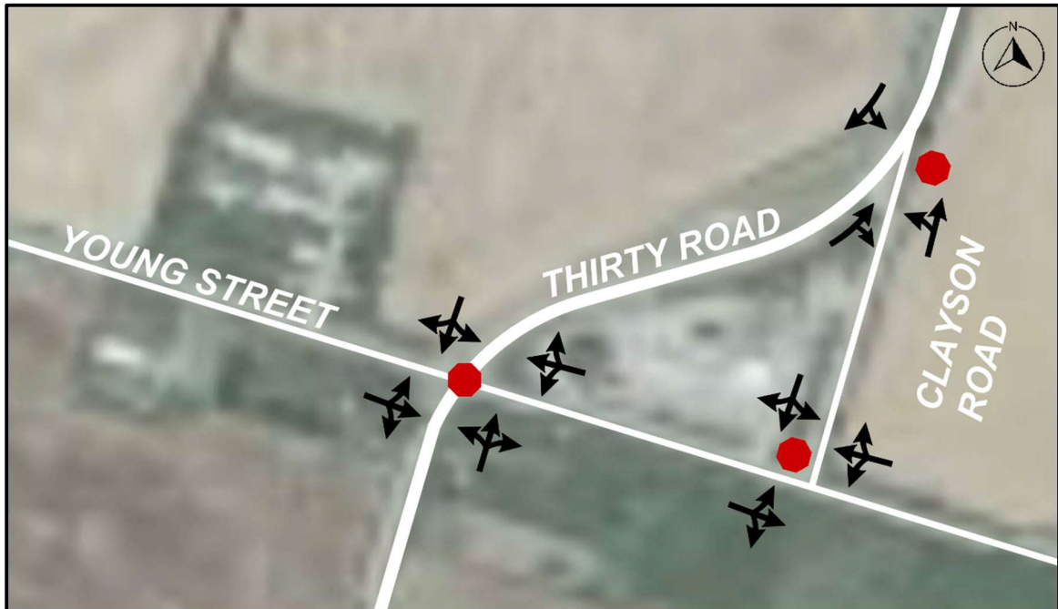
Figure 2.2 – Existing Intersection Configuration
