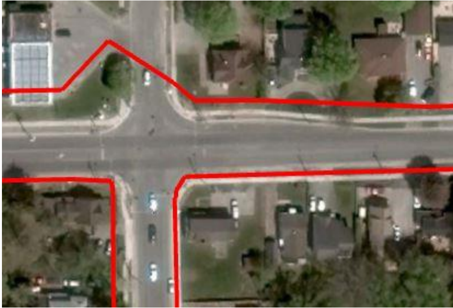
Image 12: Widened northeast corner of the Highway 20 West and Haist Street intersection for righthand turn lane in 2015
