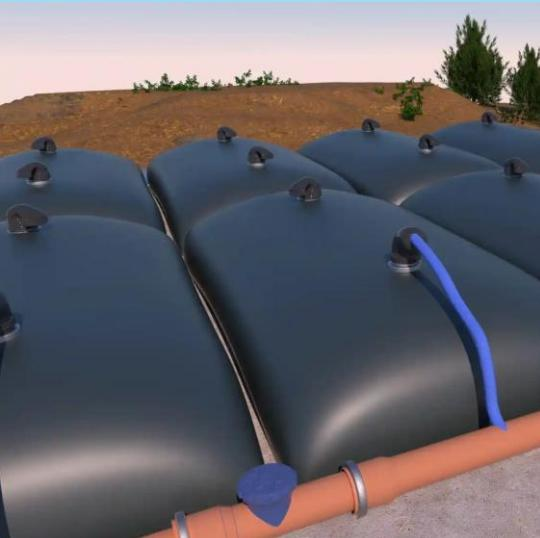
**Description:** Residuals stream is thickened, supernatant discharges back to lake, and thickened residuals are pumped to a non-mechanical dewatering process. Thickened sludge is pumped to a large geotextile filter bag (geotube). The membrane allows water to pass through, but retains the solids inside the bag. Solids that remain in the geotube are removed and disposed of at a landfill.
