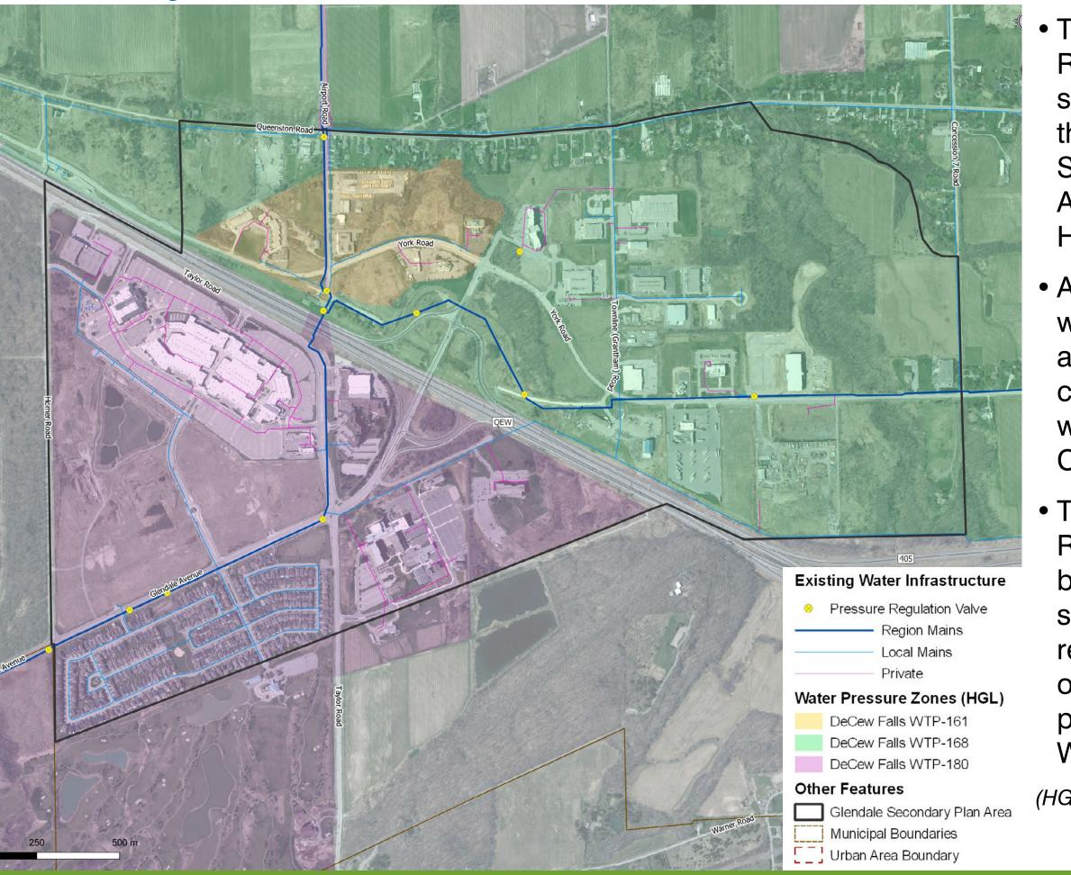
The existing and planned Region water network can supply phased buildout of the Secondary Plan Area Scenario 1 – Lower Density Assumptions and Scenario 2 – Higher Density Assumptions.
