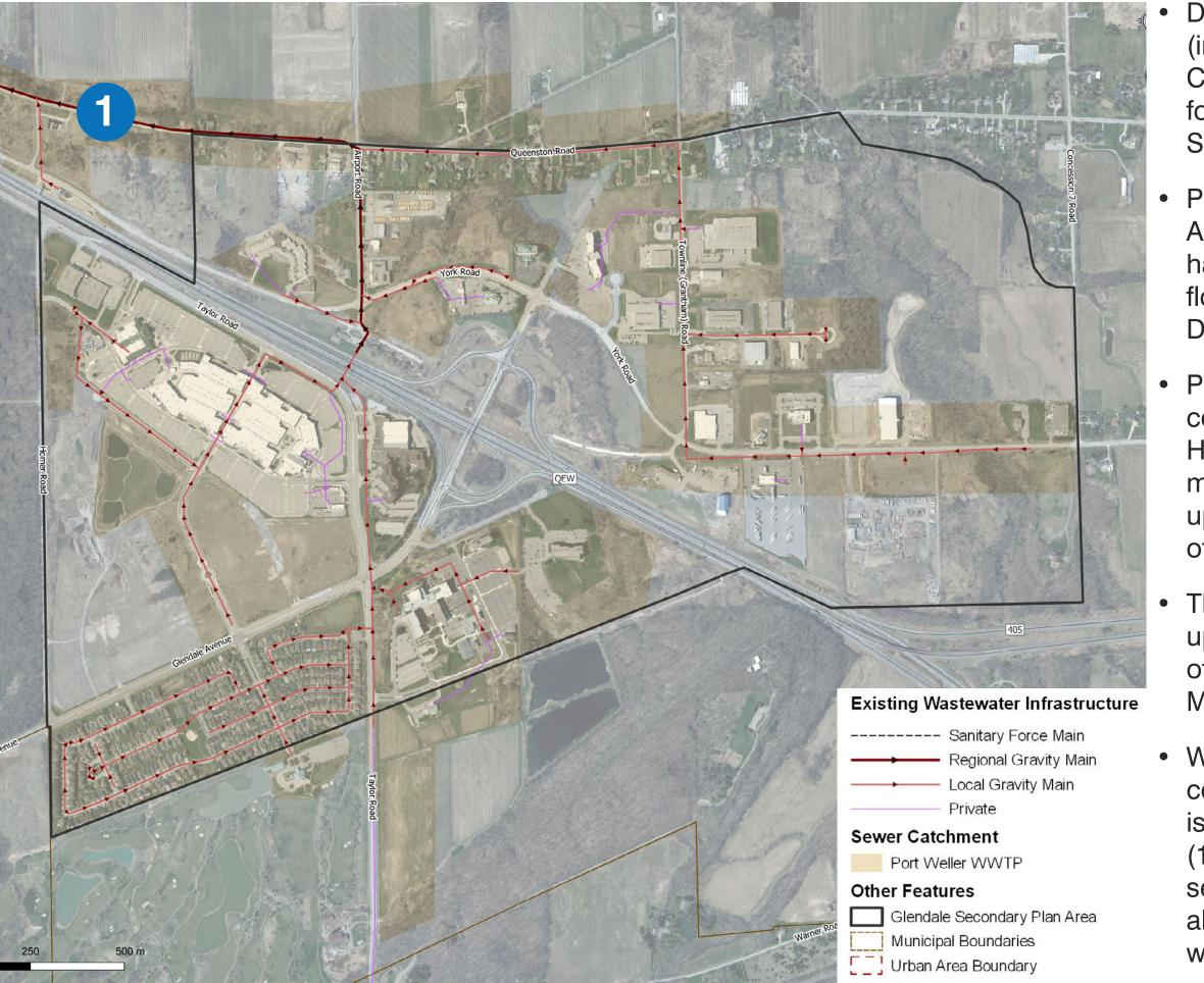
Downstream Trunk Sewer (including Siphon under Welland Canal) are to be monitored for available capacity as the Secondary Plan Area is built out.
