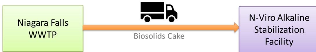
Figure 11-3: Area B Scenarios for Dewatering
