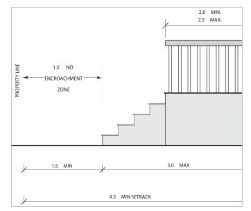
Figure: Design guideline for front porches.
