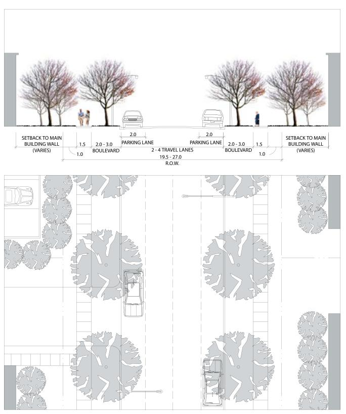
Figure: Design standards for Collector Street in an Employment configuration.
