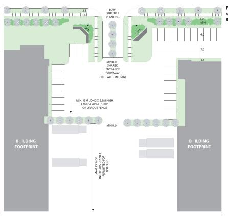
Figure: Guideline for screening of loading and service area. Landscaping should be used extensively for screening.
