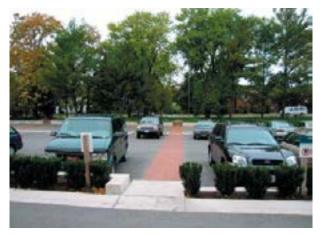
Figure: Pedestrian walkways should be provided through parking areas to enable safe and direct pedestrian movements.
