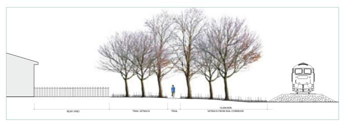
Figure: Minimum trail setback to Rail Corridor is 10.0m. This may be reduced if a safety fence is provided.
