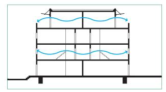
Figure: Natural ventilation systems should be considered as an alternative means to air conditioning.
