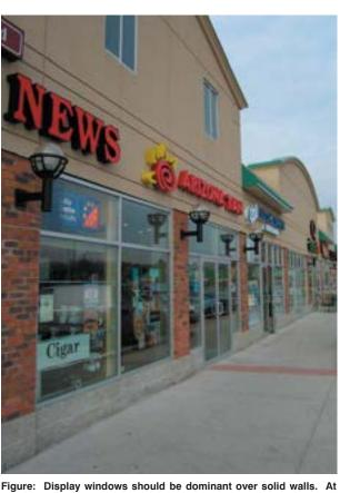
Figure: Display windows should be dominant over solid walls. At least 60% glazing should be provided at grade.
