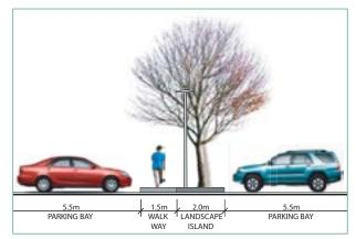
Figure: Section demonstrating preferred design of pedestrian walkways located within the parking aisle. The walkway should be a minimum width of 1.5m.
