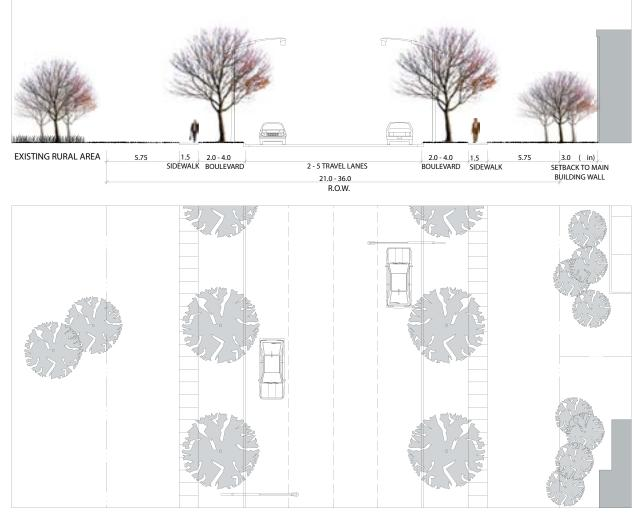
Figure: Design standards for 4-lane Arterial Road.
