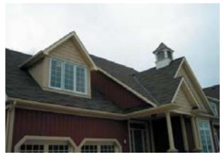
Figure: A variety of roof shapes should occur in each residential block. Where sloped roofs are required, a minimum 30 degree slope is recommended.
